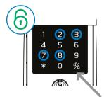
Slide cover up to energise keypad. Enter 4 digit PIN then press %
